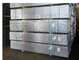
The products are manufactured from hot dip galvanized carbon steel. Purchased galvanized coils are divide into narrower bands whose width fits the specific profiles and accessories. Then, steel profiles are manufactured through roll forming technique while accessories are cut from bands according to relevant specifications.
